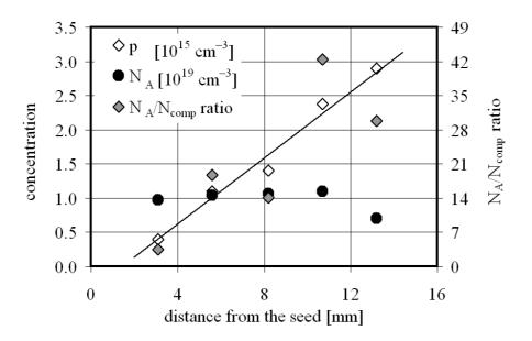
Fig. 1: Axial evolution of the charge carrier concentration p and the boron concentration  $N_A$  calculated from temperature-dependent Hall effect measurements in a boron doped 6H-SiC crystal. The charge carrier concentration in boron doped SiC samples is linearly correlated to the  $N_A/N_{comp}$  ratio while the boron incorporation stays virtually constant with growth time.
