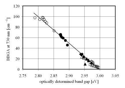
Fig. 2: Dependence of the boron-related below band-gap absorption (BBGA) peak at 730 nm on the optically determined band gap E determined by an  $\alpha^{1/2}$  / E plot according to [4]. The different symbols denote different B doped 6H-SiC crystals.
